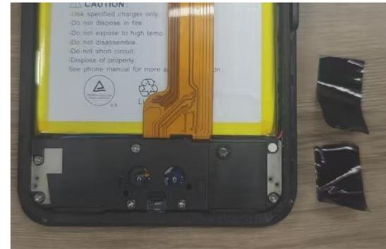
6. Remove antenna frame and speaker box frame,
