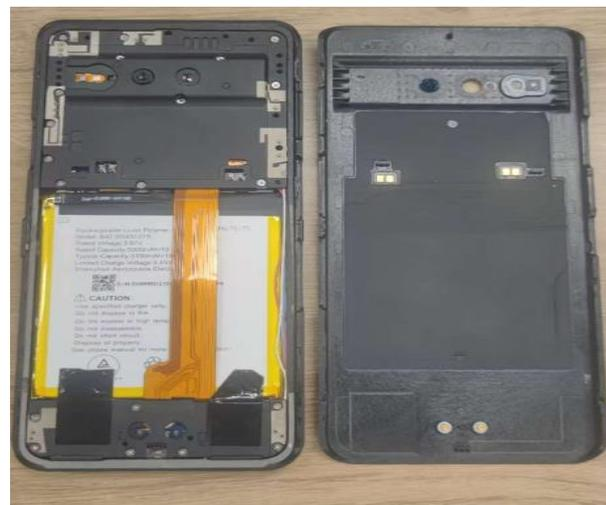
5. Disassemble 20 screws (M1.4\*5.0mm) and remove Volume key and PTT key
