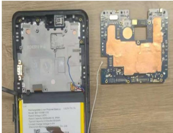
10. Remove Sub-PCBA board, Antenna PCBA and FPC
