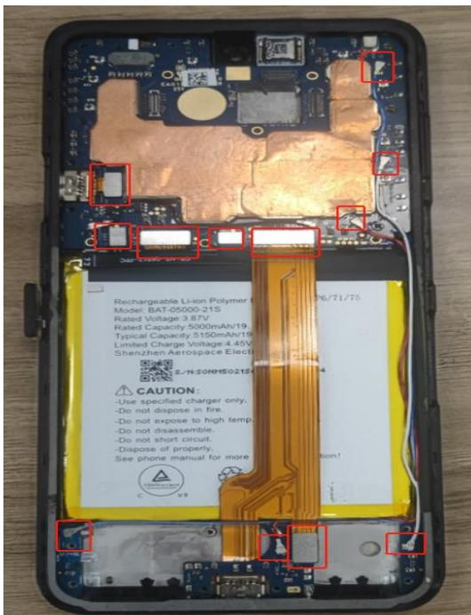
9. Unscrew 2 screw (M1.4\*2.8mm) and connectors, and then remove main PCBA board
