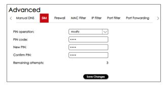
NOTE: The SIM PIN can be obtained from your service provider. If your SIM PIN has been entered incorrectly 3 times, the SIM card will be blocked – if this happens, you will need to contact your service provider to obtain a PUK code to unblock your SIM card.
