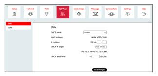
The DHCP server assigns IP addresses to all devices connecting to the H700. If required, you can modify the IP address scheme and DHCP lease time that your network will use when assigning IP addresses to devices connecting via Wi-Fi, Ethernet or USB.
