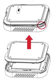
To maintain the IP68 rating against dust and water ingress, secure the protective flaps on all external ports (labelled 1, 2 and 3 on the 'Getting to know your H700' page) and ensure that the battery cover fits securely. **NOTE:** If you experience difficulty removing the battery cover, please use the provided battery cover lever tool to assist (see diagram below).
