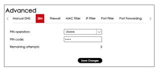
To Modify, set PIN operation to 'Modify', enter your current PIN, New PIN, then New PIN again as confirmation, the 'Save Changes'.
