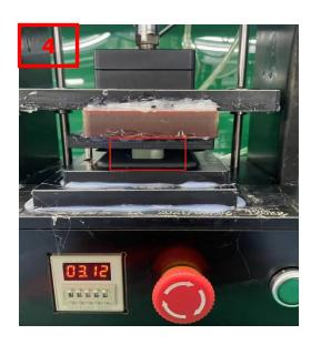
Manually or with a press and apply pressure for 12 seconds
