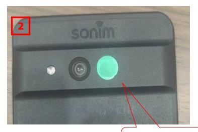
The green side of the infrared camera lens is on the outside
