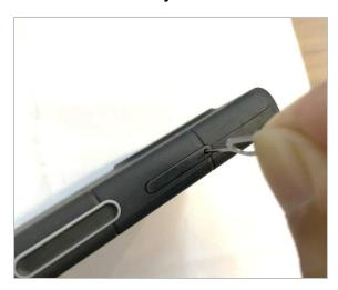
2. Remove two screws to disassemble Sub-USB cover
