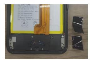
6. Remove antenna frame and speaker box frame,
