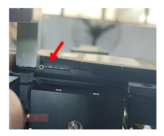
Remove Battery cover with an opening tool. (ie. iFixit tool or "black stick")
