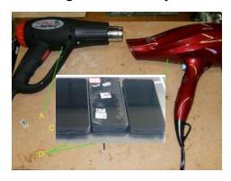
4. After heating Battery cover, separate Battery cover from Front casing.
